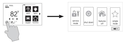
**Shut Down** - When Shut Down is selected, the OmniPL will turn off all pool equipment and report when it is safe to remove power. When this message is displayed, you can either power off the unit or restart the OmniPL by touching the large power button displayed on the left side of the screen.
