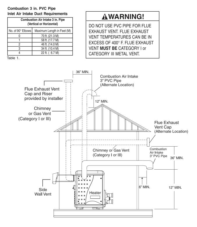
Direct Air Intake Duct with 3-inch PVC Pipe (Indoor Installation) (MasterTemp® Heater shown)
