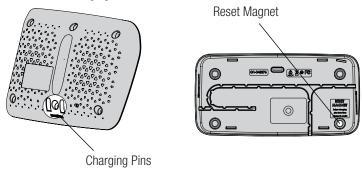
Swipe the charging pins across the reset magnet as shown below. Note that you MUST swipe from left to right and the AquaPod 2.0 will shut down. When shut down, there is no battery drain and the unit can be stored or shipped. To reboot, place the AquaPod 2.0 into the charging cradle. Note that the AquaPod 2.0 can sometimes shut down if it is subjected to a sudden shock or drop. Placing it back in the charging cradle will restart the unit.
