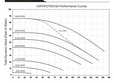
Based on independent third-party lab testing at 1725 and 3450 RPM from 6 ft.
